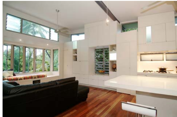
A raking ceiling with high level windows for venting hot air
